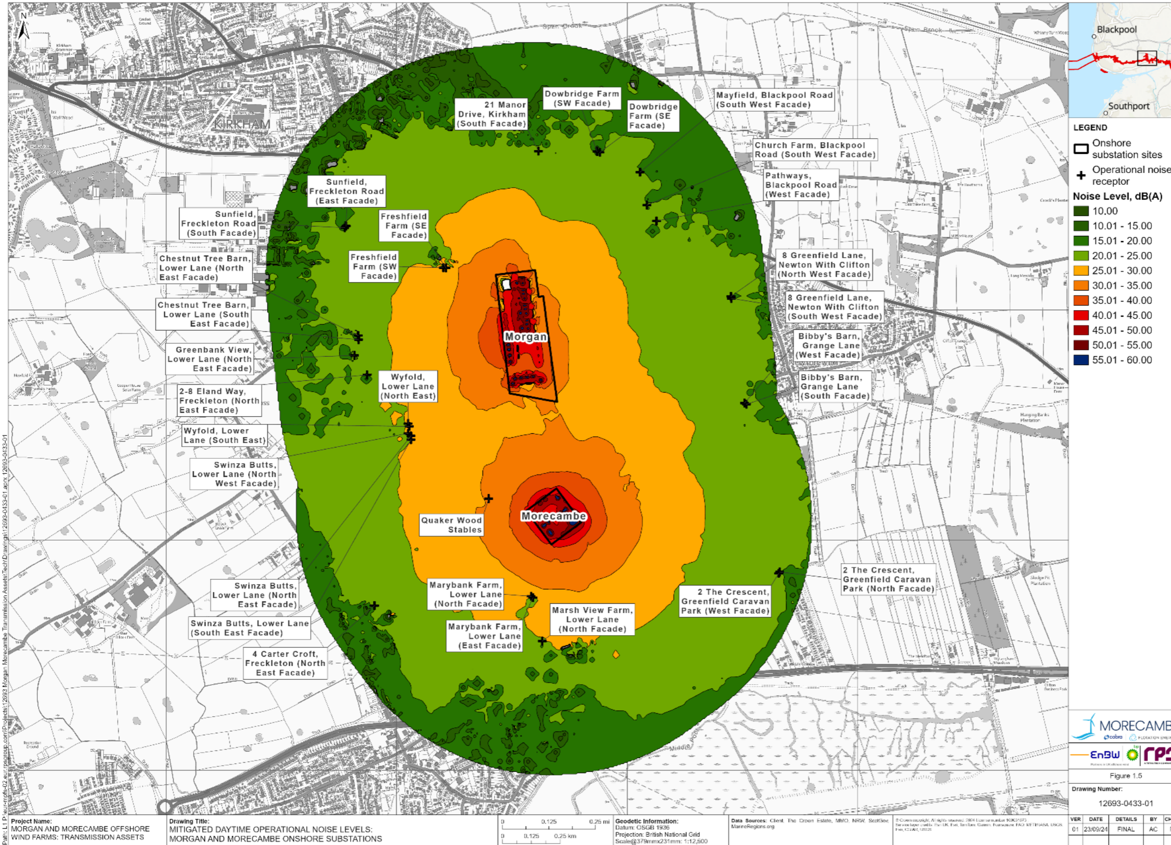
Figure 1.5: Mitigated daytime operational noise levels (Morgan and Morecambe Onshore Substations)
